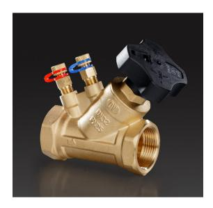
Oventrop double regulating and commissioning valves "SVTR ecQ" are installed in hot water central heating and cooling water A/C systems with a closed water circuit and serve to achieve a hydronic balancing between the various circuits of the system.
