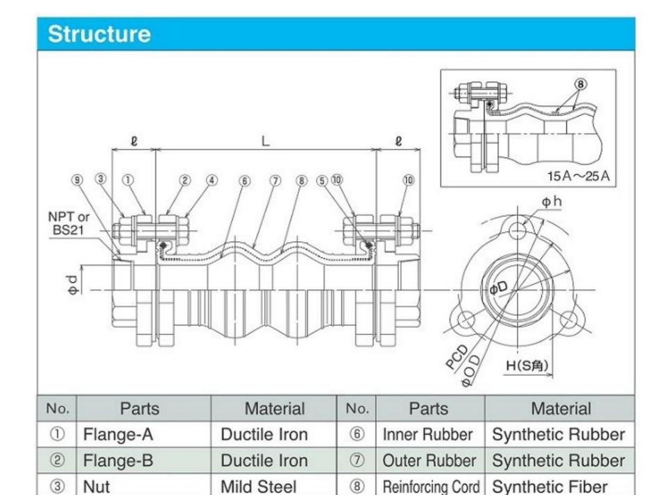
The material of No.1, 2 & 9 can be changed to SUS304 and SUS316.
