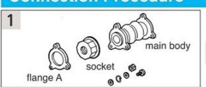
Remove the bolt and disassemble flange A and socket from the main body.
