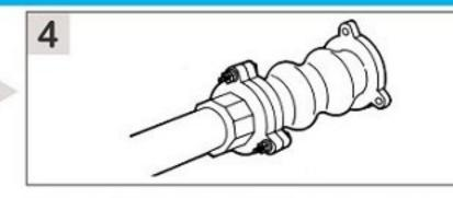
Use bolts to connect flange A and B.
